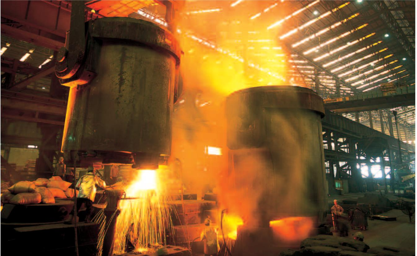
Doosan's steel foundry consists of steel-making and casting shops. The steel-making shop equipped with electric arc furnaces and ladle furnaces has a simultaneous tapping capacity of 700 tons and annual production capability of 260,000 tons of molten steel. This line also has vacuum stream de-gassing equipment to produce heavy ingots for forging and vacuum oxygen de-carburizing equipment for stainless steel.
