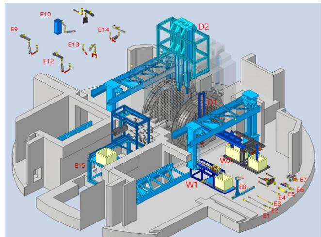
Design of Dismantling Equipment for Radioactive Structures (PHWR)
