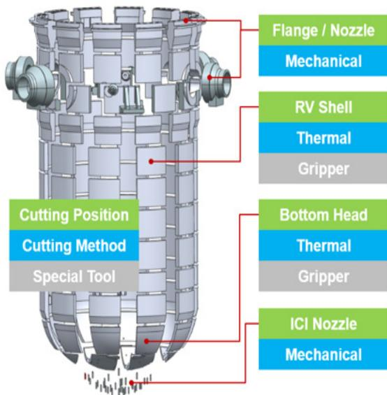
Cutting Plan & Cutting Method for RPV(PWR)
