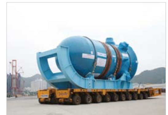
Shipment of Sanmen Nuclear Power Plant's AP1000 Reactor (July 23rd, 2011)
