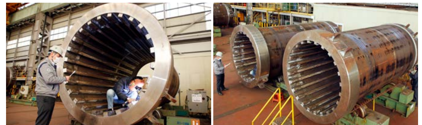
Cask manufactured at Doosan's Changwon Plant for the TMI Nuclear Power Plant in the U.S.
